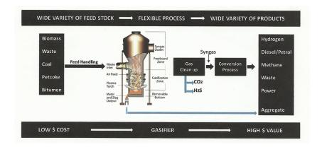
FIGURE 2. Plasma gasification process
