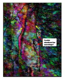
**Figure 7b:** Color blended display (z-slice at 692ms) co-rendered with similarity, more clearly resolve the major faults (F1 & F2) and a myriad of local fractures and joints.
