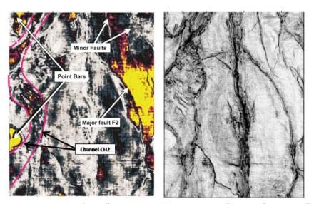
Figure 9: Horizon slice at 1424ms (a) Energy map (b) 10Hz frequency slice showing the channel outline (c) Similarity map
