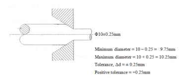
FIGURE 2. Tolerances on a particular product
