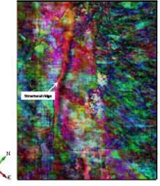
Figure 7a: RGB color blended display at horizon slice (692ms). Note the distinct difference between the northern and southern margins from the central area. Interpreted also is the NNW – SSE trending structural ridge.
