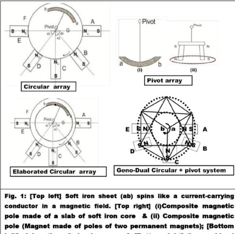
left] elaboration of circular array; & [Bottom right] the combined circular and pivot to reflect its three-dimensional cube-hexagon ("geno-dual") symmetry.
