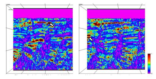
FIGURE 3. Inline 11724 and 11904 across which energy attribute have been extracted; the white arrow points toward the bright spots.
