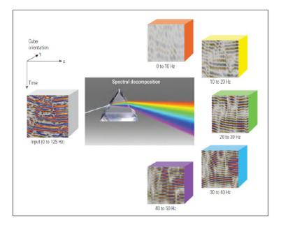
FIGURE 1. Fourier components of a broadband seismic pulse (After Aarre et al., 2012).
