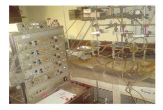
FIGURE 1. Grass Polygraph Model 7D Recorder and Organ Baths. The aortic rings are suspended in an array of organ baths which can record from 3 to 4 rings simultaneously
