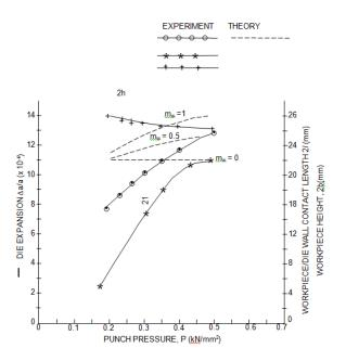
FIGURE 12. Plots of die expansion against punch pressure
