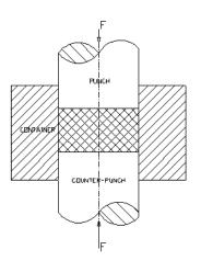
FIGURE 3. A completely closed cavity die
