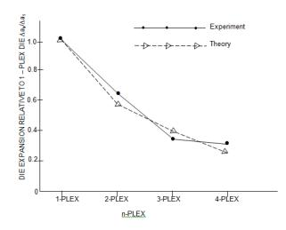
FIGURE 13. Plots of die expansion against degree of die compounding
