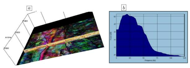
Figure 8: Three iso-frequencies of the seismic bandwidth around the zone of interest (8b) blended in the RGB display (8a).
