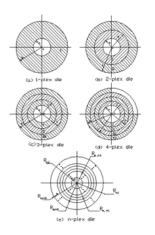
FIGURE 8. Selection of degree of die container compounding
