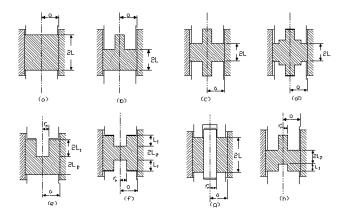
FIGURE 5. Closed cavity die forging
