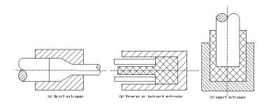
FIGURE 6. Extrusion processes
