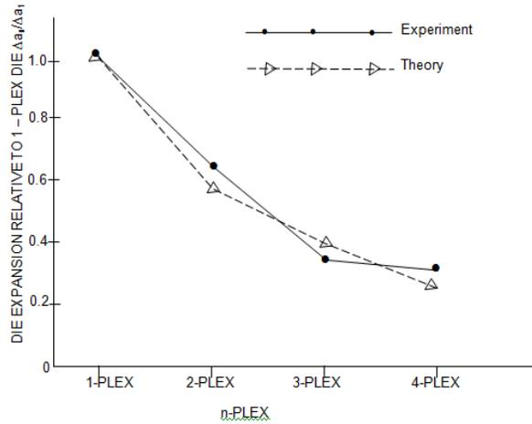
FIGURE 13. Plots of die expansion against degree of die compounding
