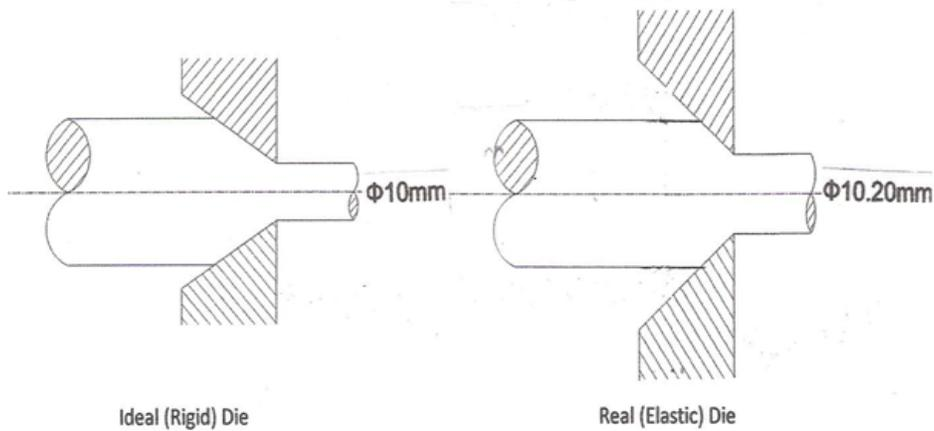
**FIGURE 1. Comparison of ideal (rigid) and real (elastic) dies under same impressed load**
