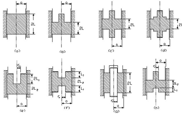
FIGURE 5. Closed cavity die forging
