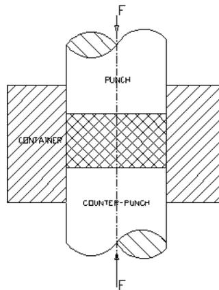
FIGURE 3. A completely closed cavity die
