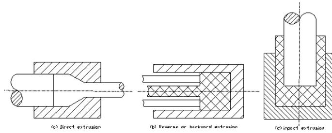
FIGURE 6. Extrusion processes
