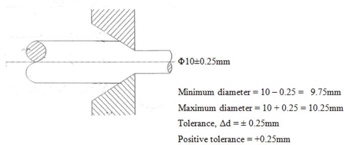
FIGURE 2. Tolerances on a particular product
