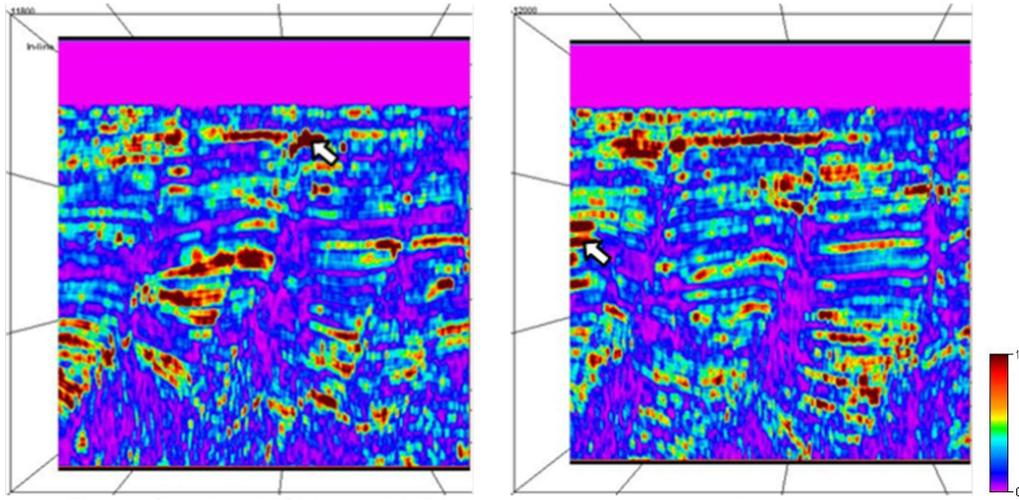
FIGURE 3. Inline 11724 and 11904 across which energy attribute have been extracted; the white arrow points toward the bright spots.
