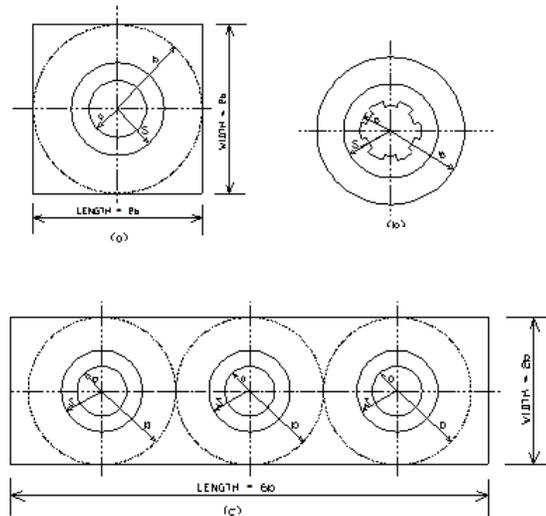
FIGURE 4. Extension of the design method to other forging dies
