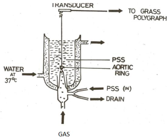
FIGURE 2. Schematic diagram of an Organ Bath. The aortic ring is suspended between a hook at the bottom of the bath and a Force transducer above and perfused with Physiological Salt Solution (PSS) at  $37^{\circ}C$  bubbled with  $95\%O_2-5\%CO_2$  gas mixture. The Force transducer is connected to the Grass polygraph to record tension developed by the ring during experimentation
