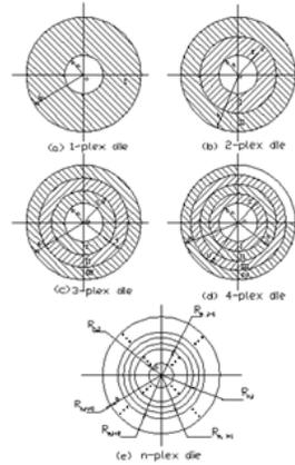
FIGURE 8. Selection of degree of die container compounding
