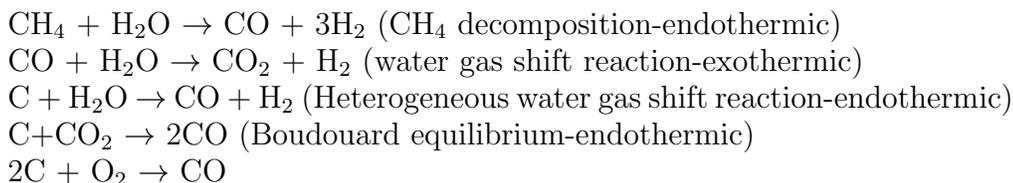
The  $H_2$  and  $CO$  generated during the gasification process can be a fuel source. Therefore, plasma gasification process has been combined with many other technologies to recover energy from the syngas.
